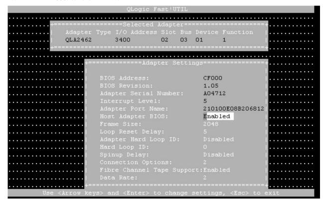
FIGURE 11-3 HBA BIOS Screen for Enabling Boot From the FC LUN
