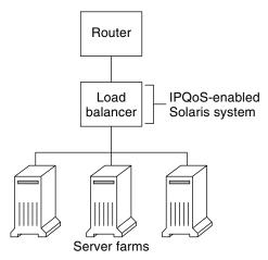
In such a topology, the router is Diffserv aware, and therefore able to queue and rate both incoming and outgoing traffic. The load balancer is also Diffserv-aware, and the server farms are IPQoS enabled. The load balancer can provide additional filtering beyond the router by using selectors such as user ID and project ID. These selectors are included in the application data.
