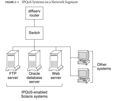
This network is but one segment of a corporate intranet. By enabling IPQoS on the application servers and web servers, you can control the rate at which each IPQoS system releases outgoing traffic. If you make the router Diffserv aware, you can further control incoming and outgoing traffic.
