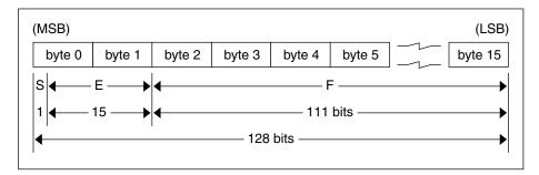
Just as the most-significant and least-significant bytes of an integer are 0 and 3, the most-significant and least-significant bits of a quadruple-precision floating- point number are 0 and 127. The beginning bit, and most-significant bit, offsets of S, E, and F are 0, 1, and 16 respectively. These offsets refer to the logical positions of the bits, not to their physical locations, which vary from medium to medium.
