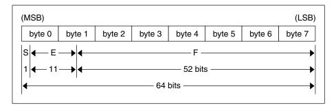
Just as the most and least significant bytes of an integer are 0 and 3, the most-significant and least-significant bits of a double-precision floating-point number are 0 and 63. The beginning bit, and most significant bit, offsets of S, E, and F are 0, 1, and 12 respectively.
