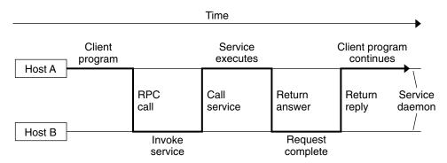
An RPC is analogous to a function call. Like a function call, when an RPC is made, the calling arguments are passed to the remote procedure and the caller waits for a response to be returned from the remote procedure.
