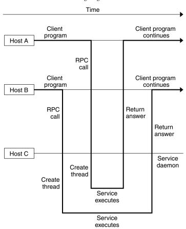
FIGURE 7-2 MT RPC Server Timing Diagram
