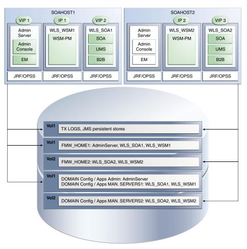
Figure 4–2 Example Configuration for Shared Storage
