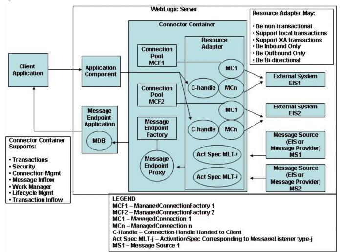
Figure 2-1 Connector Architecture Overview
