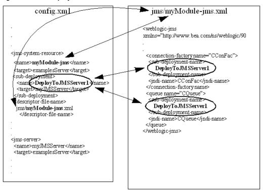
Figure 7-1 Subdeployment Architecture
